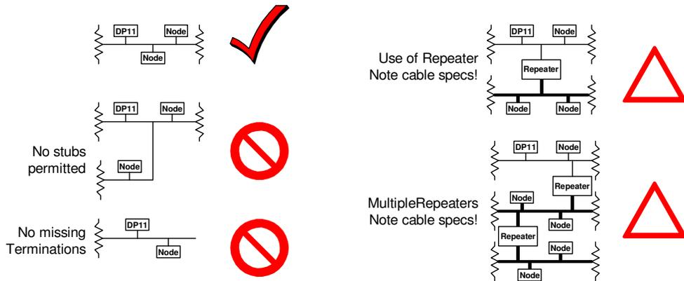
Figure 1 RS 485 Cabling Topologies
